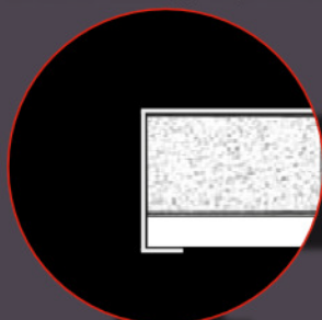
18 gauge steel wrap around end caps
